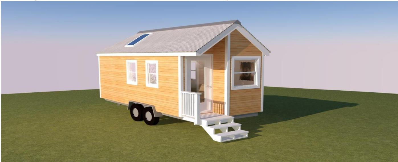
The SPARK **Bondy 15** is a 6 Meters long tiny house on wheels with a 10/12 gable roof. It has a bathroom sized to fit a square shower stall, composting or standard toilet, and small wall mounted sink. A small kitchen could be placed in the center of the house. A sleeping loft above the bathroom & kitchen space provide enough space for a queen sized mattress. Two skylights and a small window open to provide ventilation in the loft.
