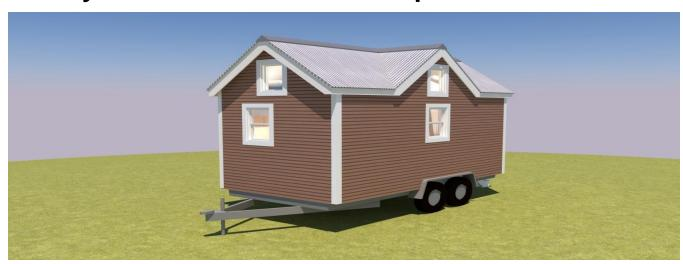
The SPARK **Creek 12** is a 4.8 Meters long tiny house on wheels with a 10/12 gable roof. It has a bathroom sized to fit a square shower stall, composting or standard toilet, and small wall mounted sink. A small kitchen could be placed in the center of the house. A sleeping loft above the bathroom & kitchen space provide enough space for a queen sized mattress. Two skylights and a small window open to provide ventilation in the loft.
